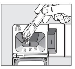
The horizontal marks in Compartment II indicate levels of approximately  $1 \frac{1}{4}$ ,  $1 \frac{3}{4}$  and 2 tablespoons (20, 25 and 30 ml) respectively.
